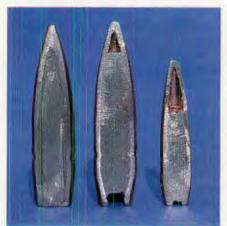
A comparison of sectioned projectiles (left to right): 148 gr. LPS, 152 gr. 7N1, 60 gr. 5.45x39 commercial load. Notice the steel core of the LPS round is surrounded by lead. With the 7N1 the steel core sits on top of a lead knocker. The air cavity in the nose is similar to that used with the 5.45x39 to increase leathality.
